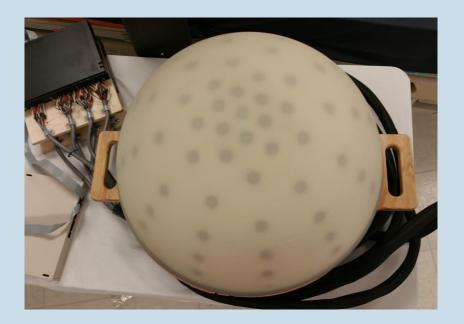
Immersion (high resolution) and Envelopment Sensor vertical spacing is ¾", horizontal varies Shows envelopment More than actual pressure Pressure by sensor row , more rows is better
